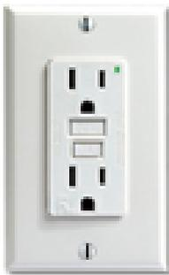
shorted out you could get seriously hurt or killed before the breaker would open. That's where the GFI's come in. A Ground Fault Interrupter will open a circuit almost instantaneously when it detects current going to anywhere other than through it, so as to prevent injury. That is why they are required in wet places like kitchens, bathrooms and garages. Your outside outlets should also be on a GFI. When a GFI senses about a 5 milliamp (.005 of one amp)
