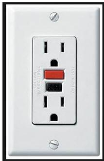
kitchen outlets are on a ground fault interrupter (GFI) circuit. However, they are not always in the same room. There may be one GFI for both bathrooms and the outside outlets are usually protected by the ones in the garage. This may or not be the case so locate all your GFI's so you know where they are. When you find them, test them by pressing the test button and then the reset button.
